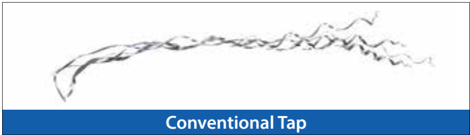
Chip generated in 40m/min
